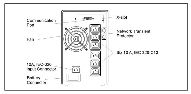
Figure 3. PW5125 1000i and PW5125 1500i Rear Panel
